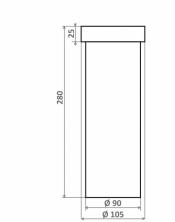
Number of LEDs 36 Type of LEDs 120° SMD LEDs (S) Warm white 2700K (F), Warm white 3000K (E), Neutral Color(s) white 4000K (N), Cool white 6000K (W), Red (R), Amber (O), Green (V), Blue (L)
